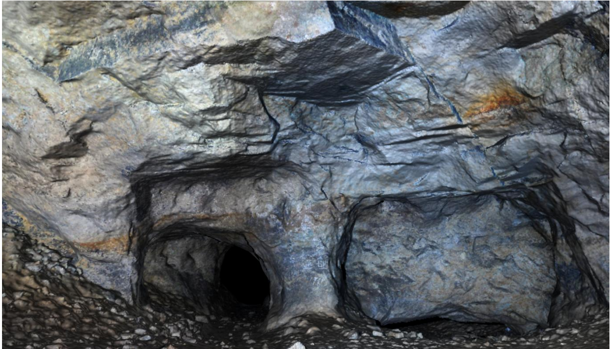
Fig 1: Terrestrial lidar derived 3D model of faulted and fractured sandstones within the West Mine
